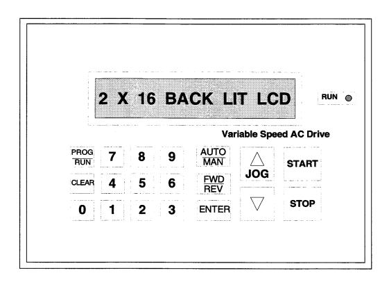
When the drive is first powered up it will be in the operating mode in standby. The display will appear as follows:
